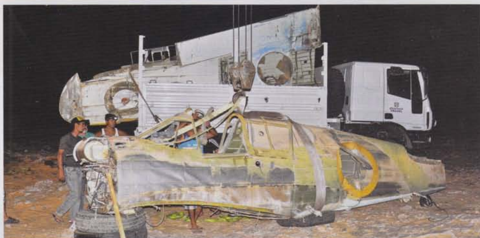
Wings safely stowed, the fuselage is prepared for lifting onto the deck of the light truck.
