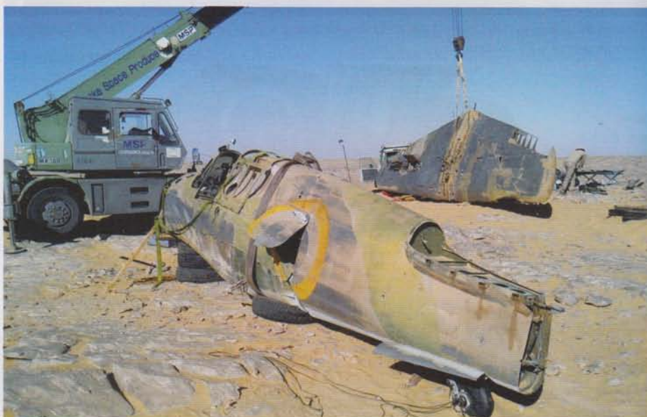
Success! The wing (background right) is positioned for further disassembly. Following removal of the wing centre section fuel tanks, the wing was separated along the centreline by undoing the connecting bolts.
