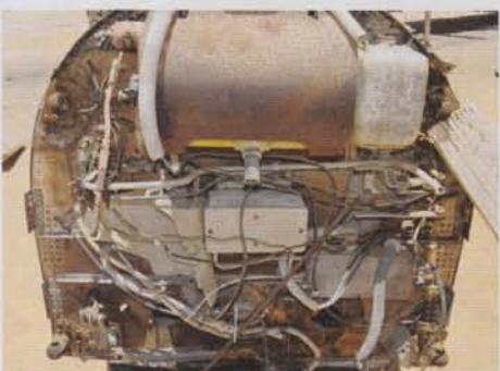
Forward of the cockpit and the firewall is the oil tank, containing 13.9 US gallons (49 litres).
