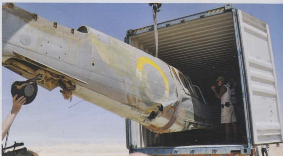
The fuselage back was broken and as a result had to be very carefully hoisted by positioning the fuselage lifting straps forward of Frame 9.
