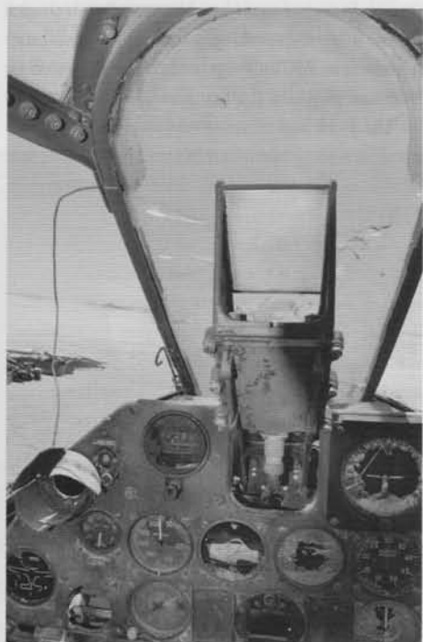
Cockpit view of the reflector gun sight and armoured windscreen. Note cracks in the latter, the result of Egyptian Army soldiers firing rounds into it.
