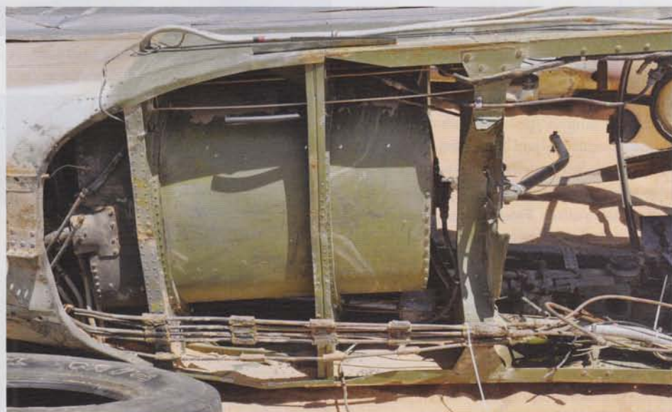
View of the aft cockpit fuel tank. Capacity is 62.5 US gallons (236.6 ltrs). The team have checked the fuel tank, cables and connections to ensure nothing would be crushed once the fuselage was loaded into the container.
