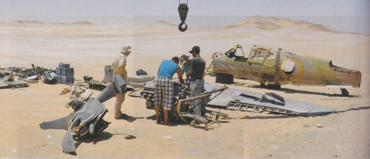
Around two miles (3.2 kms) from the crash site the Allison V-1710 engine is prepared for loading onto the container truck. The wrecked propeller is in the foreground.
