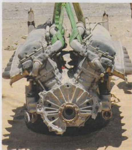
Close up of the Allison, showing the damage where the reduction housing has been ripped off during the crash landing.
