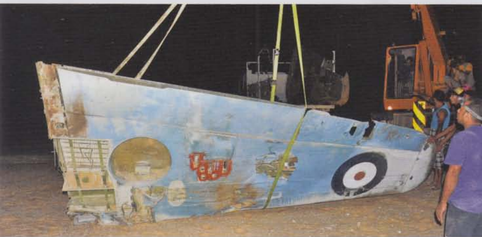
The underside of the starboard wing protected from UV light for seven decades reveals its Azure Blue paint and remnants of the US applied Sky Blue.
