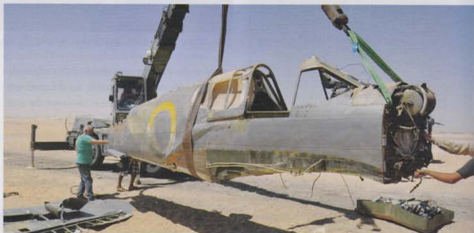
The fuselage back was broken and as a result had to be very carefully hoisted by positioning the fuselage lifting straps forward of Frame 9.
