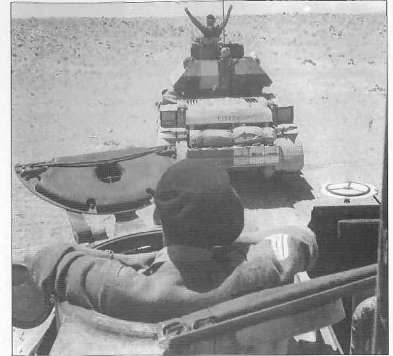
Late April 1941: hand signals signifying 'Advance' from an A13 Cruiser Mk II tank of 5th RTR. Note the sun-compass mounted close to the nearer tank commander's right elbow – see photo on page 3. (IWM E 2639)
