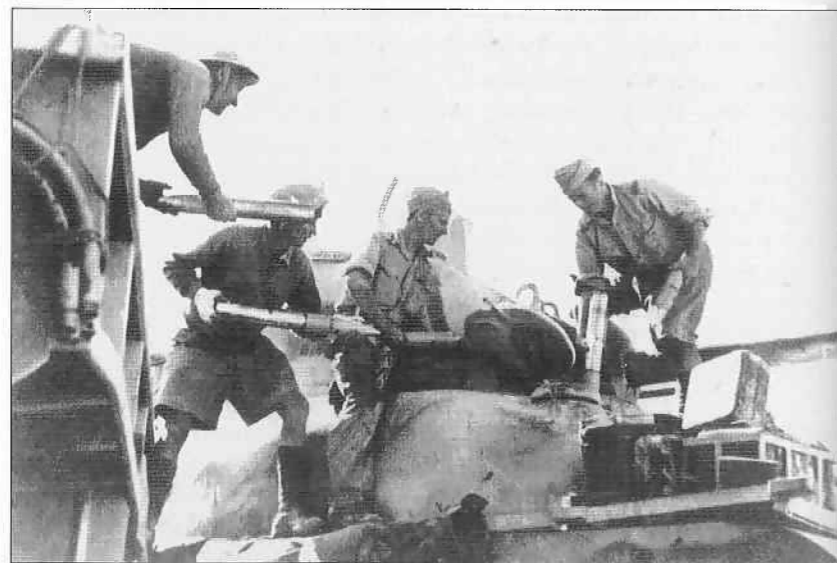
Re-ammunitioning a Sherman of 9th Lancers from a supply truck. The Sherman – supplied to this unit of 2nd Armd Bde, 1st Armd Div just in time for Second Alamein – had thicker armour than previous types, a more reliable engine and running gear, and the great tactical advantage of a high mounting for a 75mm all-purpose gun. The harder work of handling the larger and heavier 20lb shells was a light price for the crew to pay, even though the Sherman was designed to carry no fewer than 90 rounds. (Private collection, courtesy Mike Chappell)
