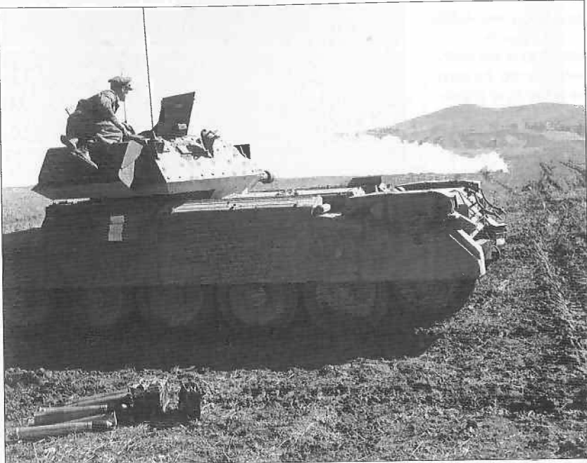
Le Kef, Tunisia, 12 February 1943: Crusader tank of First Army testing 6-pdr smoke shell – see Plate E. Ever since 1916 British tacticians had set great store by smoke, and in North Africa they had practised with it rather more often than they were able to use it in combat. Before the arrival of the Grant tank in spring 1942 it usually had to be fired from field artillery, but smoke shells would become increasingly available for tanks from mid 1942 onwards. The sporting cry of ‘Two up and bags of smoke!’ (i.e. two units forward, one in support) would only increase its hold upon the British military imagination thereafter. (IWM NA 785)
