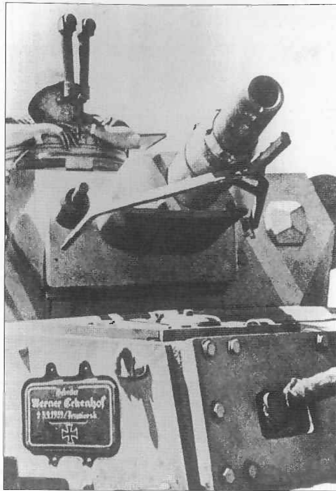
Turret of a PzKw IV with the short 7.5cm gun, showing a binocular rangefinder in use. One of the Germans' tactical advantages lay in their superior optical instruments, which helped them to deliver accurate fire at long ranges; typically the PzKw IV would fire HE from around 2,000 yards. The British eventually realized that they were being 'out-telescoped', which only reinforced their feelings of inferiority when faced by DAK Panzers. However, in desert conditions even the best optics were often frustrated by the dust that vehicles threw up, or by the distortions created by heat hazes; the hottest part of the day, in mid afternoon, was often a very difficult time to fight a battle. Note the memorial plaque to a dead crewman, painted over the vision slot beside the bow MG-gunner's position. (Tank Museum 7417/A4)
