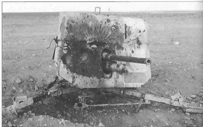
Knocked-out British 2-pdr (40mm) AT gun, shot square through the gunshield during the post-'Crusader' fighting in December 1941. The damage appears to have been done by a 5cm AP shell, which might have been fired by either a towed AT gun or a PzKw III. The 2-pdr should have been replaced by the much more powerful 6-pdr (57mm) during 1941, but the production programme was set back a year by the losses incurred in France in 1940. The first 6-pdr AT batteries would arrive only for the battle of Gazala in May 1942. (IWM E 7060)
