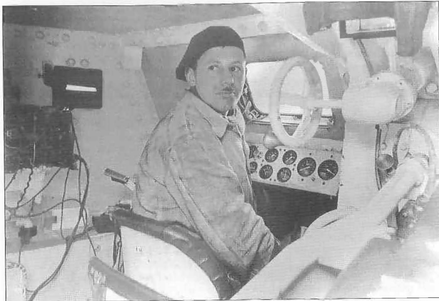
Driver's compartment in a Grant tank – see Plate G insets. The unusual hull design of the M3 Medium made this surprisingly spacious. Note the radio transceiver behind his left shoulder, and his large open front visor. This might seem enviable compared with those of other tanks; but it did let in a lot of blowing sand when on the move, and when closed down for action the driver had to peer through the usual tiny, disorienting vision slit, like that to his left. (Tank Museum 2729/E2)
